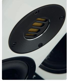
The Jet 5 tweeter vibrates a very light, finely pleated foil to project high frequencies
