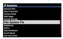
If you try using storages formatted with non-commercial version of NTFS driver(old version firmware) with the X40 new firmware, the X40 may not detect it properly at first booting, and say 'Query Error'. In this case, please try running 'File System Fix' at SETUP
