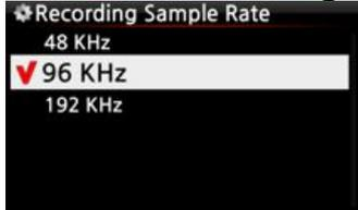
When you record by X30, you can set Recording Sample Rate by one (1) of three (3) options like 48Khz, 96Khz, 192Khz.
