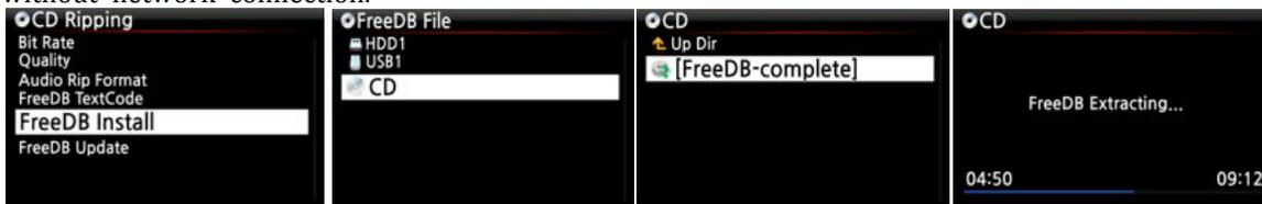
To install the FreeDB data to the X30 hard disk, insert the FreeDB data DVD into the CD slot of the X30 and go to SETUP and select FreeDB to install. You will see the CD, select and confirm with the OK button. The X30 will shut down and reboot to start installing the FreeDB data automatically.
