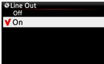
In case that you want to use an external amplifier, the line out (Analog Out) should be set as ON, and the external amplifier should be connected to the line out (analog out) at the rear of the X30.
