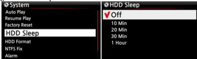
For the X30 to wake up from HDD sleep mode, it takes 3~4 seconds. During this time, the X30's response to the input signal from remote control will be delayed.
