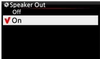
When you want to use the amplifier of the X30, the speaker out should be set as ON
